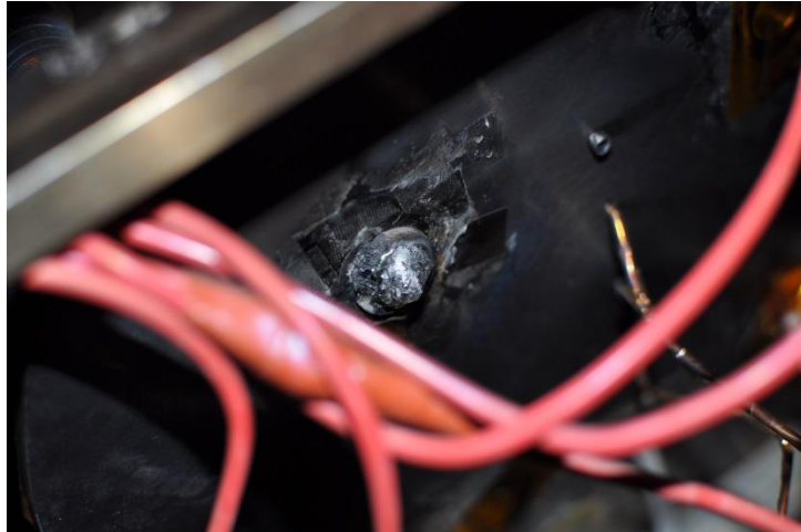
Fig. 45. The results of plasma attaching to an anode support on the backside of the P5—a mildly deformed 6-32 nut and bolt.
