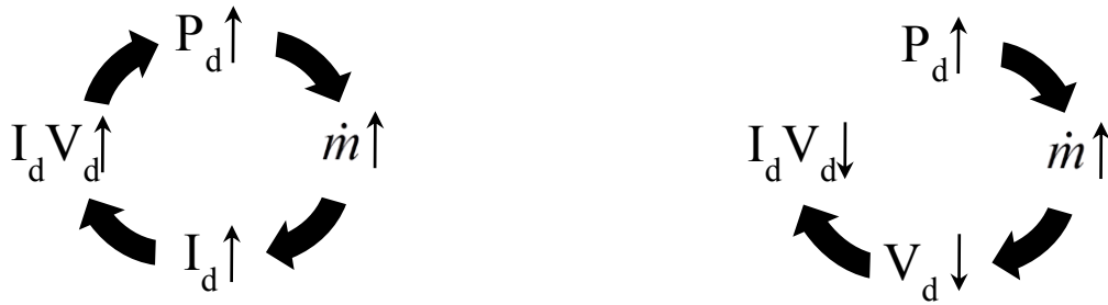
Figure 1. Left: Voltage-limited operation resulting in run-away current. Right: Current-limited operation arrests runaway mass flow.
