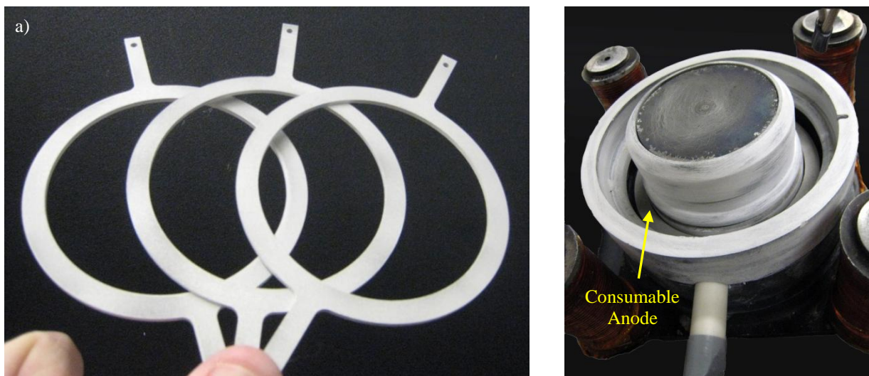
Fig. 4. Images of a) three consumable magnesium anodes and b) a single magnesium anode inside the discharge channel of the thruster with the front plate and BN ring removed.
